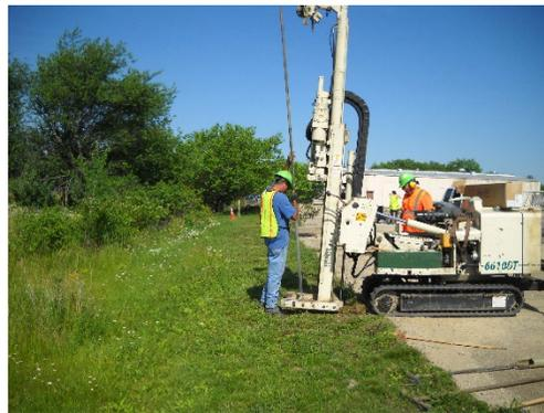
Figure 3: Direct Push Technology Drill Rig
