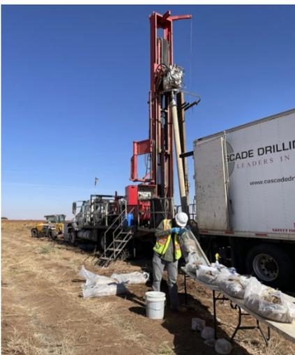
Figure 2: Sonic Drill Rig
